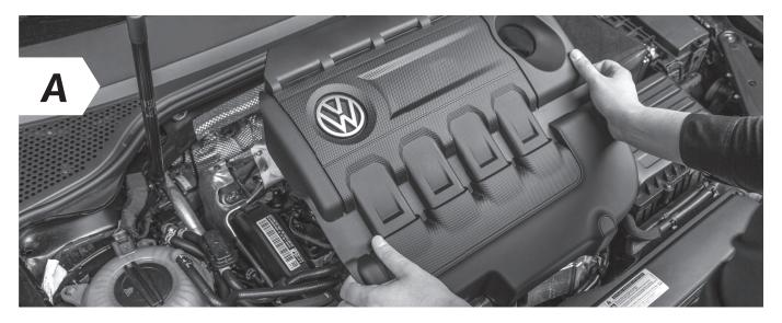
• Remove the engine cover and place it next to the car. You may have to jiggle the cover slightly to release it from the holding clips.
