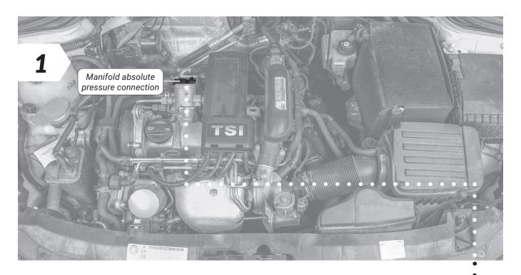
Once the connection to the turbo boost pressure is complete, it is time to make the connection to the manifold absolute pressure.
