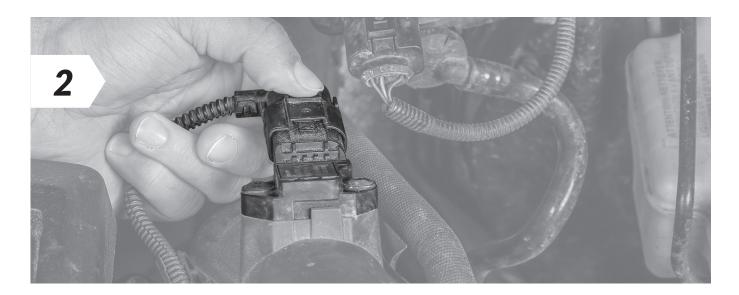
Disconnect the plug from the turbo boost pressure sensor.
