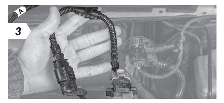
• Now connect the end of the RaceChip wiring harness marked "A" to the disconnected connector and the other end to the sensor.
